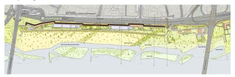
Figure 6.32. The Vistula River Park – conception of reconstruction of goyne's system located on right bank of the river between two bridges: Lazienkowski and Poniatowski (Damiecki et al. 2008)
