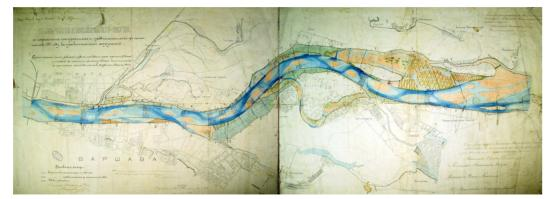
Figure 6.8. The project of the Vistula River training works made by Kostanecki in 1873, executed by Lindley in 1884 – 1889 as a part of the water supply infrastructure project in Warsaw (Damiecki i in. 2008).
